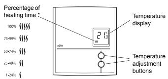
\* The thermostat displays the percentage of heating time required to maintain the desired temperature. For example, §§ is displayed when heating is activated 40 percent of the time.
